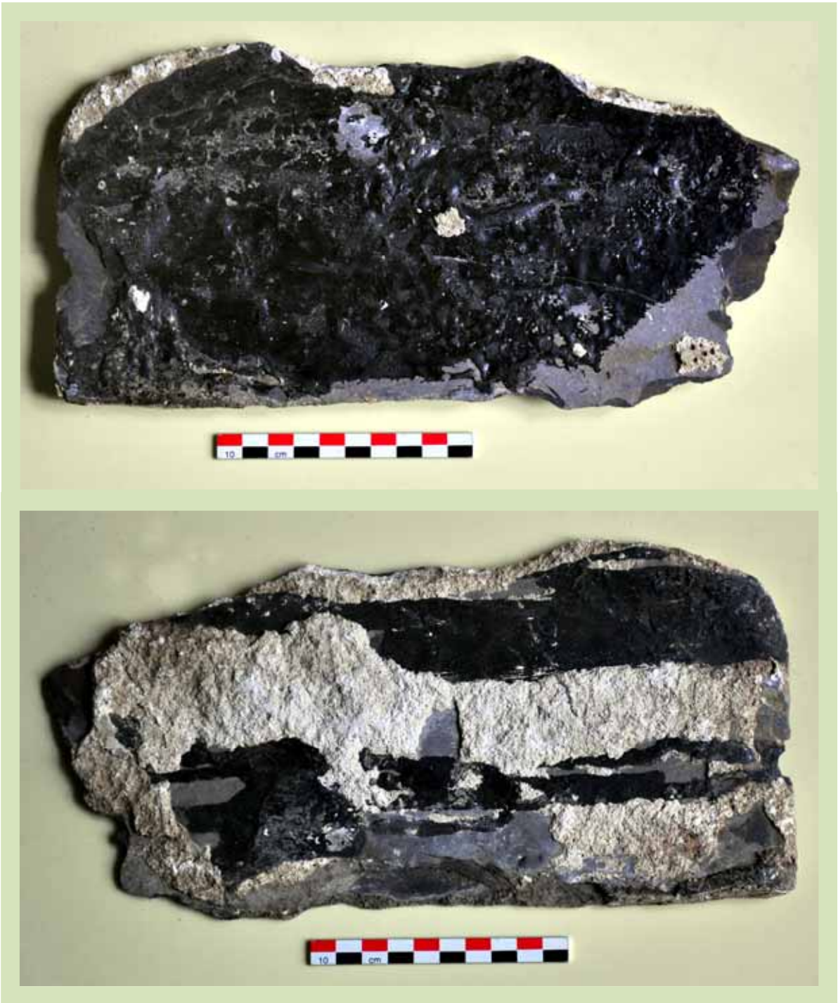
Figure 2. Slate fragment with lime mortar and bitumen. AGT 03 BM 11. (ph 0920 & 0921)
